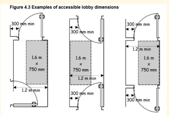
Where either door can be secured by a locking device, the lobby should be not less than 1.5m wide. This will permit a wheelchair or pram to be turned around should passage be denied.
